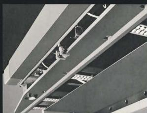
This device supports the worksheet and keeps it from sagging while it is being pushed into the shear. When shearing is completed, the electromagnets are turned off automatically and the sheared blank falls onto the chute. Residual magnetism is not retained in the worksheet.
