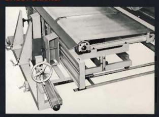
This unit carries cut sheets on a conveyor and automatically stacks them at the rear of the shear. Scrap is automatically separated by using a selector switch at the front of the shear.
