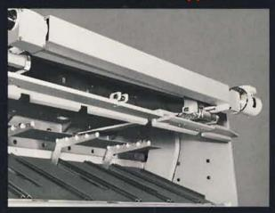
This device is most convenient when shearing thin non-magnetic material. The support bars have plastic rollers so that the worksheet will not be damaged or scratched. An air supply is necessary for this device.
