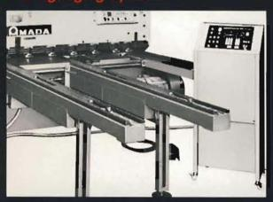
This is an NC controlled front gauging system. Front gauge positions can be selected by data input through the numeric keypad. The worksheet is correctly positioned by pushing it firmly against the front gauge stops.
