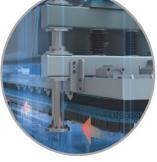
◆ Deburring block belt. The block is using abrasive flap/nylon or steel wire or abrasive filament for various application. Edge rounding for the edge sharp parts after wide belt grinding. Combination of top and bottom function. Even and efficient edge rounding on side and edges.
