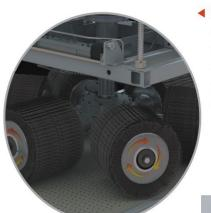
■ Wide belt grinding unit and planetary type deburring unit. Used for the surface finishing and burrs removal for the sheet metal punching and cutting parts. No sharp edges. No burrs left on the holes. Perfect deburring for the film coated work piece and coating sheet.
