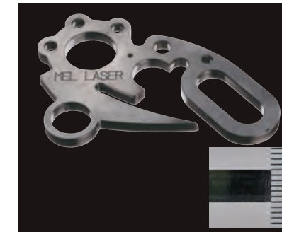
Material/Thickness: Mild steel (SS400) t6mm
