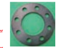
Processing Shape Material: Thickness: Mild Steel t25mm Assistgas: Oxygen
