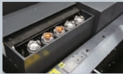
Nozzle changer These features reduce setup time and support system automation while maximizing productivity.
