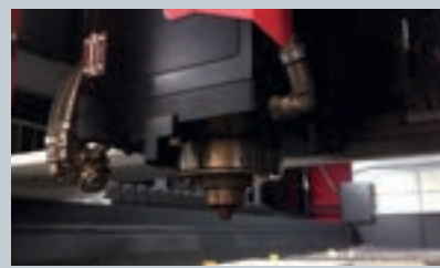
High Peak Piercing Reduces piercing time for mild steel processing.
