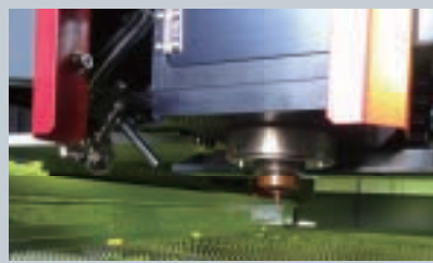
Oil spray function Reduces spatter adhesion when piercing during mild-steel processing.
