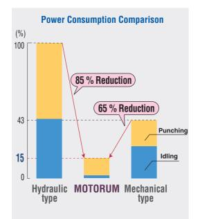
Energy efficient machine design enables a drastic reduction in machine running costs and conservation of natural resources.
