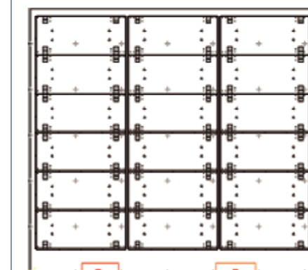
Worksheet example (SPCC/1.2 t) Material size: X1250mm × Y1000mm Number of tools: 6 Total hits: 660
